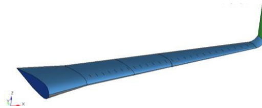
Fig. 4. Meshing of wing without vortex generators
